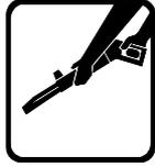
The spray lance is affected by a thrust during operation - therefore always hold it firmly with both hands. **IMPORTANT: Point the nozzle at the ground.**
